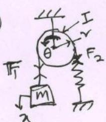
$$F_1 = -m\ddot{x}; \quad F_2 = Kx; \quad (F_1 - F_2)r = I\ddot{\alpha} = I\ddot{\theta} = I\frac{\ddot{x}}{r}$$
