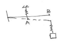
Deflection of wars at B due to Spring Ki = (Porce at A due to Mg)/K, = (mg x a)/K, Deflection due to k, at B = (mg 1/a) x \( \frac{1}{4} = mg (4a)^2 \) Total deflection at B = D, due to ky + Azdue to tr  $\Delta = \frac{Mg(Ma)^2 + \frac{Mg}{k_2}}{k}$  $\omega = \sqrt{\frac{9}{\Delta}} \Rightarrow \sqrt{\frac{K_1 k_2}{M(K_1 + K_2(1/\Delta)^2)}}$
