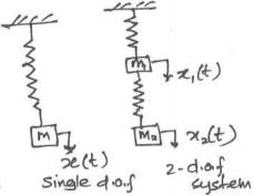
The number of independent parameters needed to describe are 2. Hence this is called a two degrees of freedom system. Similarly if two rotors are mounted on
