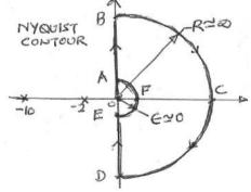
Note: Poles of GH are the roots of the denom. of GH. Poles of GH are also poles of (1+GH)
