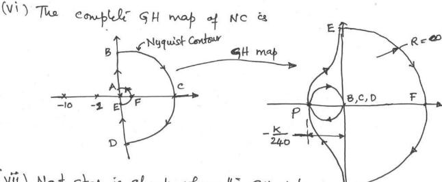
(VII) Next Step is check where the GH plot A ceets the real axis. If it ceets to a point to the right side of (-1,0), then the number of encirclements of (-1,0) will be zero. So that N = Nz-Np or Nz = N+Np, from which Ng the roots of chave equi, 1+GH=0, lying in the right half place can be evaluated. If NZ +0, then the C. Egn. has roots with positive real parts, and system would be unstable.
