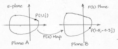
Each point s in plane A (called s-plane) is mapped to a point in plane B (called the F(s) map in this case). We map each point on A, moving in CW or CCW direction, to points in B. The path in B will also be closed.
