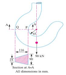
19) A crane hook has a round cross section with diameter 95mm. The bed diameter is 125mm. (a) Determine the load which will produce a maximum stress of 125 N/mm² in the inner fibers; (b) Determine the load that will produced the corresponding stress in the outer fibers.
