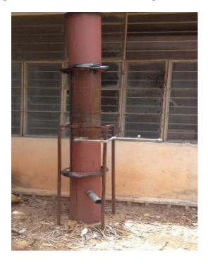
11. Design and fabrication of solar water distillation plant.
