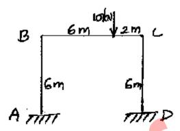
14. Draw SFD and BMD of the given continuous beam using Kani's method of analysis.
