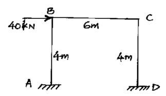
13. Draw the BMD and show all important features of the diagram using slope deflection method for the given portal frame.
