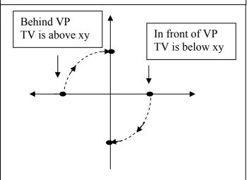
Now, using these above simple rules, just mark the points at the given distances from xy.
