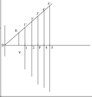
5) With Centre as F & Radius =1-1', cut arc on line 1-1' above and below to get P<sub>1</sub>, P<sub>1</sub>'. Similarly get the other points using 2-2', 3-3', etc. Join all points from V to get the required hyperbola.
