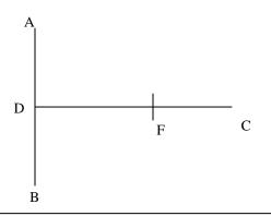
Divide DF into 3+2=5 parts. Mark V at (Divide DF into (m+n) no.of parts. Mark
