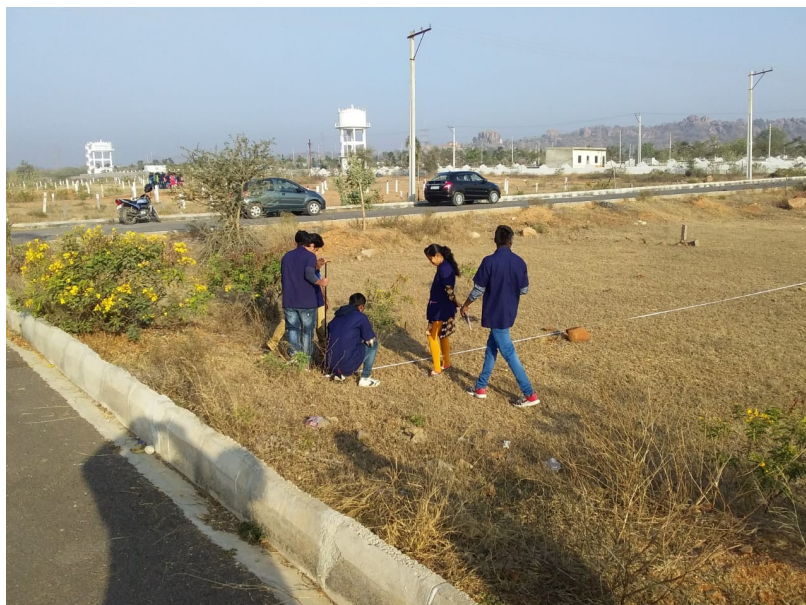
Figure 6 Students fixing the grid points for indirect method of contouring
