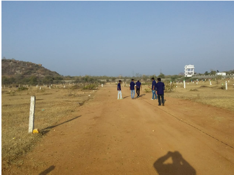
Figure 8 Students chaining center line of given alignment for longitudinal section and cross section levelling
