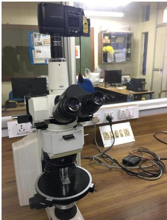
They are projected onto the monitor behind connected to this telescope and then the grain model, size, composition, colour of various elements present in it are identified.
